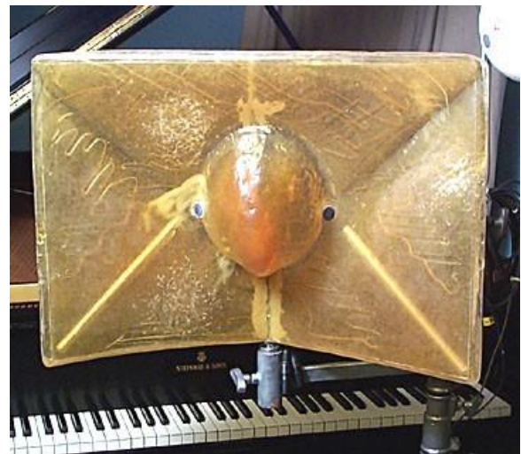
Fig. 2 Ambiphone Prototype Before Placement of Omni Capsules Within the head
